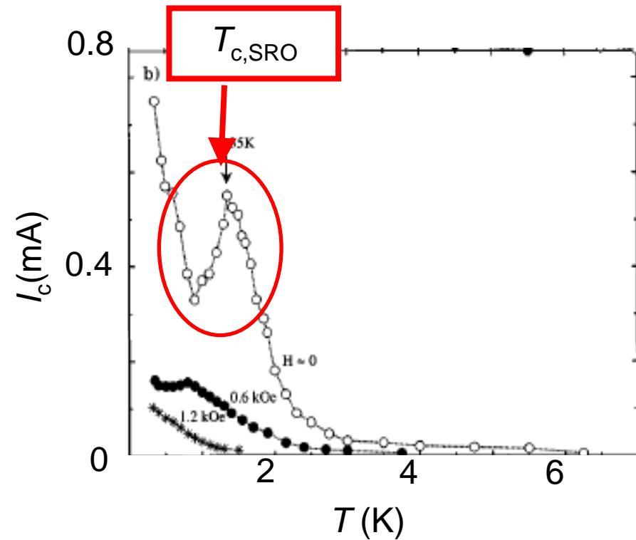
The critical current  $I_c$  is suppressed just below  $T_{c,\text{SRO}}$
